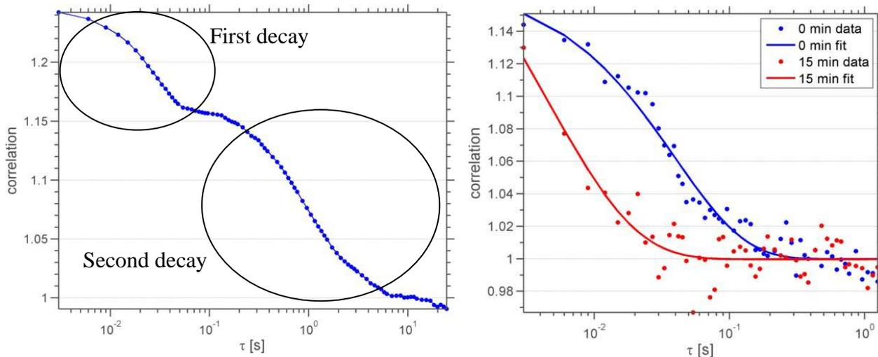
Figure 2: Left: Correlation function of OMCA-CTAB mixture after 25 min irradiation at  $q=0.025\text{nm}^{-1}$ . The two different time constants are clearly visible. Right: Comparison of the fast decay for 0 min (black curve) and 15 min (red curve) UV-irradiation duration. An influence of the UV excitation on the fast dynamics of the OMCA-CTAB mixture is evident.
