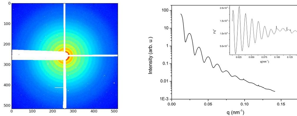
Figure 1: Left: SAXS image of the CTAB-OMCA mixture with silica particles. Right: Radial integration of the SAXS image. The position of the maxima of the curve point to the expected particle sizes of about 500 nm using the formular of the Schultz distribution.
