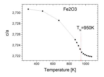
Fig.1. Ratio of the hexagonal unit cell parameters c/a of  $\alpha$ -Fe<sub>2</sub>O<sub>3</sub> determined from SR powder diffraction data. The dotted vertical line shows the Neel temperature  $T_N$ =950K.
