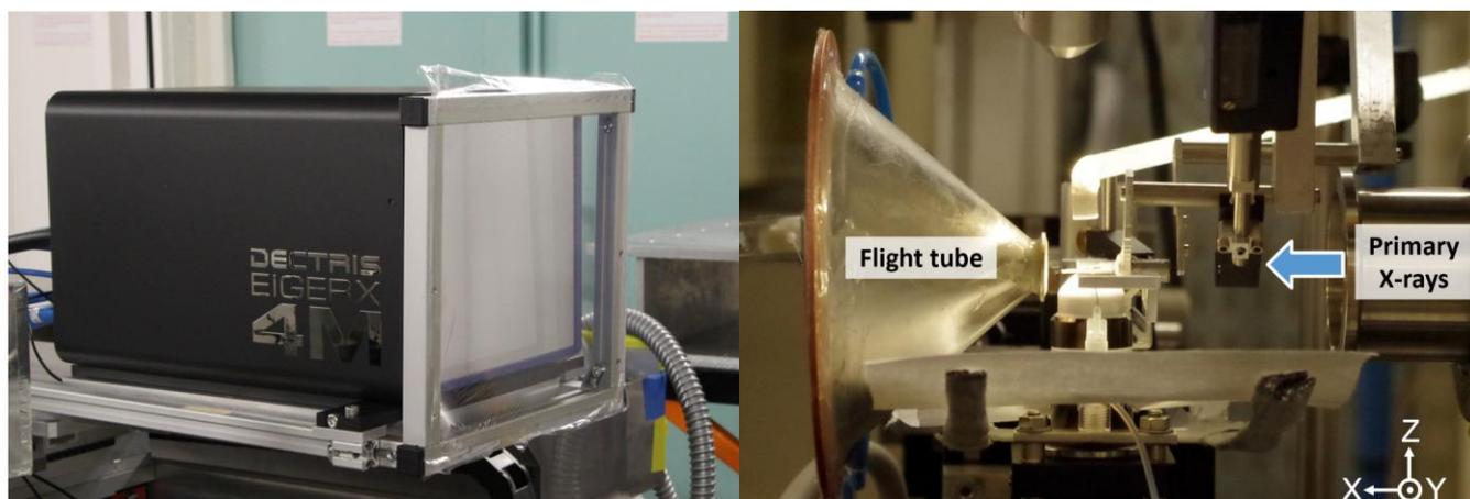
Figure 1. Photographs of the DECTRIS EIGER 4M detector installed at ESRF-ID13 (left) and the integrated flight tube flushed with helium gas to reduce the absorption and scattering by air [3] and hence resulting in improved scattered data quality (right).
