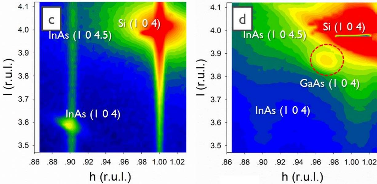
**Figure 3.** (a) and (b), SEM pictures of sample D and E, respectively. (c) and (d), RSM of corresponding samples. To highlight the InAs diffraction, the color scales are varied within these contour plots. Diffraction points are demonstrated in white text, reciprocal unit vectors are in Si substrate lattice.
