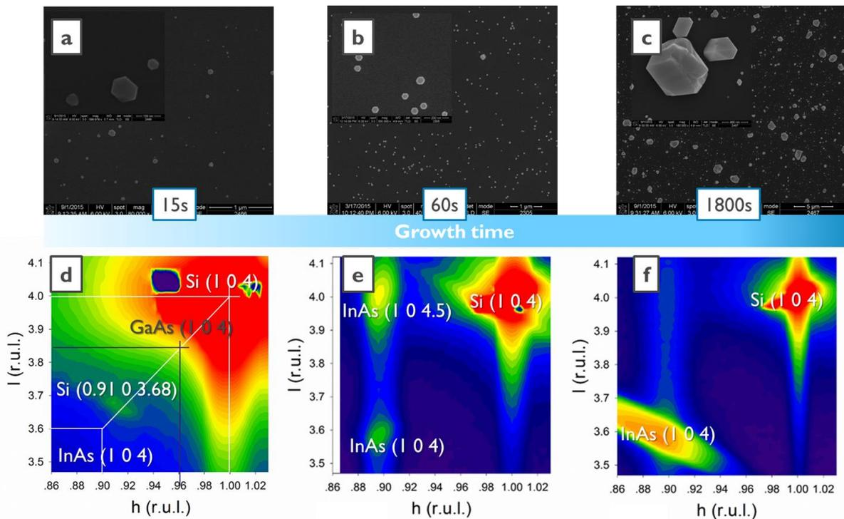
**Figure 1. (a-c) SEM pictures of sample A, B and C, respectively; higher resolution pictures are shown as insets. (d-f) RSM of corresponding samples, To highlight the InAs diffraction, the color scales are varied within these contour plots. Diffraction points are demonstrated in white text, GaAs (1 0 4) are also shown in (d) as a reference for analysis. Reciprocal unit vectors are in Si substrate lattice.**
