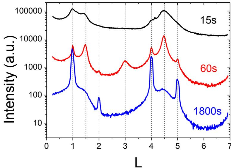
**Figure 2. InAs (1 0  $l$ ) CTR scan of sample A, B and C, plotted in black, red and blue, respectively.  $l$  is taken under InAs lattice.**
