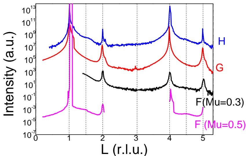
**Figure 5. InAs (1 0  $l$ ) CTR scan of sample F, G and H, plotted in black, red and blue, respectively. All are conducted in incident angle of 0.3°. F is also measured using incident angle of 0.5°, which is plotted in purple.  $l$  is taken under InAs lattice.**
