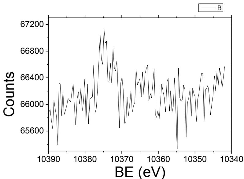
**Figure 6. Ga 1s XPS spectrum using photon energy of 14972 eV.**
