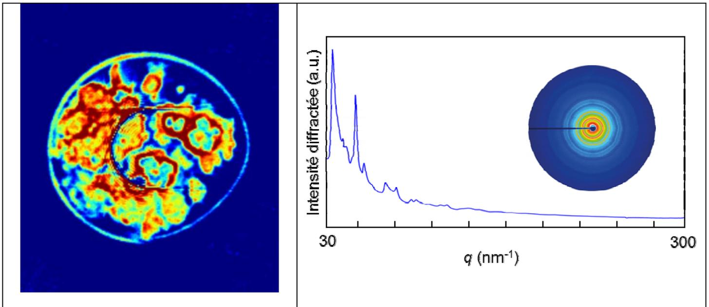
Figure 1: Analysis of the manganese nodule. Left: reconstruction of the image for a given value of  $q$ . Some intensity artefacts persist (we are working on this issue, which should be solved by writing a software that allows for data normalization). Right: XRD pattern obtained for a given position inside the nodule.
