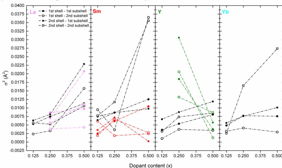
**Fig. 3.** First shell mean square relative displacement  $\sigma^2(\text{Å}^2)$  of single-doped samples for the Ce-edge (black lines) and for the rare earth (RE) edges (colored lines).
