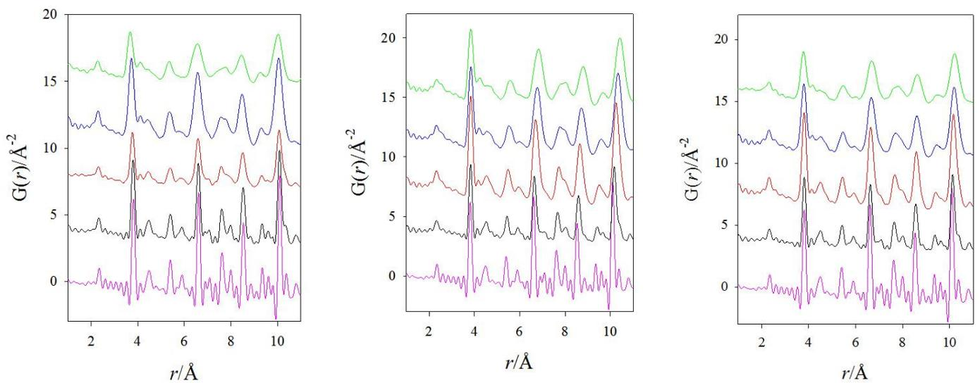
Fig. 4.  $G(r)$  function of the  $\text{Ce}_{1-x}\text{Yb}_x\text{O}_y$  (left),  $\text{Ce}_{1-x}\text{La}_x\text{O}_y$  (middle),  $\text{Ce}_{1-x}\text{Yb}_{x/2}\text{La}_{x/2}\text{O}_y$  (right) samples. Pink, black, red, blue and green lines refer to  $x=0, 0.125, 0.250, 0.375$  and  $0.500$  samples respectively
