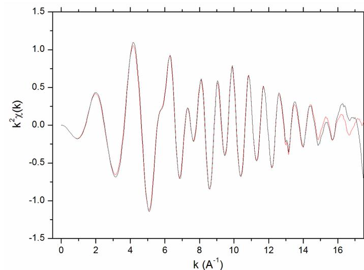
**Fig. 1.** Comparison between the EXAFS signal extracted after averaging 15 scans (red curve) and 5 scans (black curve).
