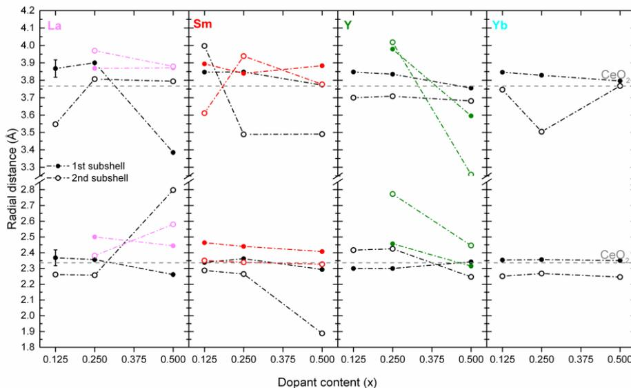
**Fig. 2.** First (lower) and second shell (upper) interatomic bond lengths of single-doped samples for the Ce-edge (black lines) and for the rare earth (RE) edges (colored lines), as a function of doping.
