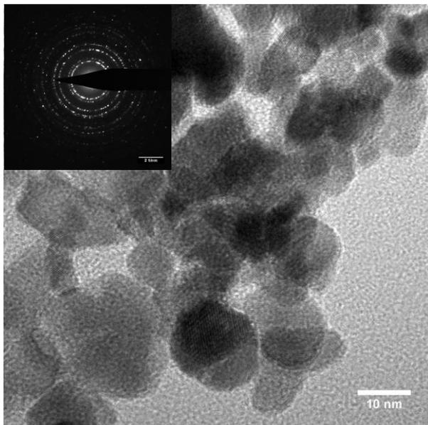
**Figure 3.** HRTEM images and electron diffraction patterns of  $\text{PuO}_2$  nanoparticles from sonochemical colloid.
