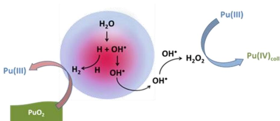
**Figure 1.** Suggested mechanism of the sonochemical plutonium colloids formation.
