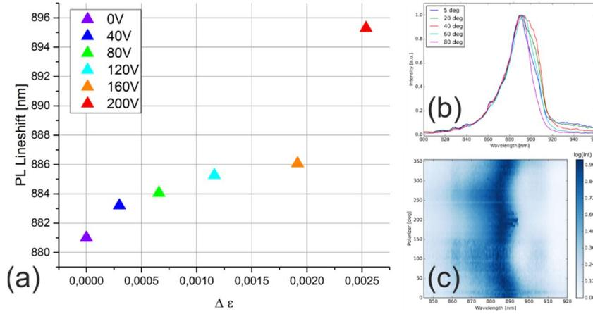
Figure 3: (a) XEOL line shift of the GaAs emission line as a function of in-plane strain. (b) XEOL spectra for different polarizer settings, showing the composition of the emission of two lines with different polarization. (c) full map of XEOL spectra as a function of polarizer angle.
