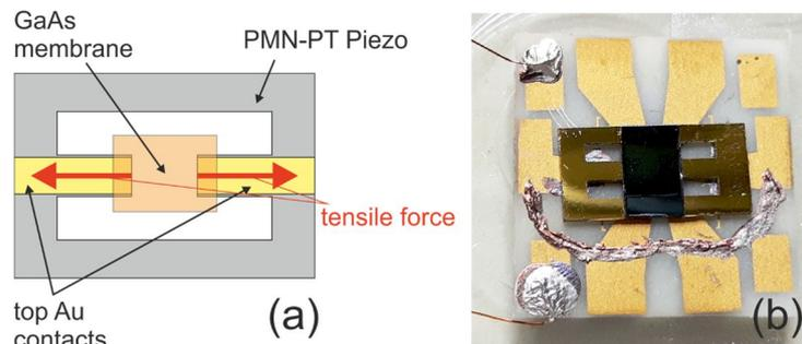
Figure 1: (a) sketch and (b) image of the two-leg piezo device to apply uniaxial strain to a GaAs membrane bonded on top. The back side of the piezo has Au contacts as well, serving as ground.
