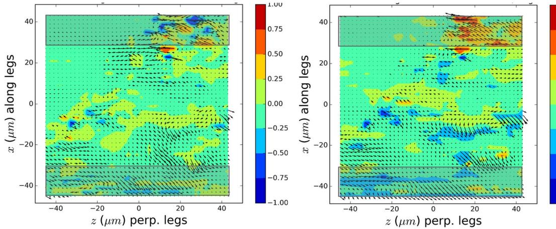
Figure 5: in-plane distribution of the strain change (colormap, in %) and tilt change (arrows; length in  $^{\circ}$  exaggerated by a factor of 2) relative to the 0V case (Fig. 4) for applied bias of 120 V (left) and 240V (right). Shaded areas show regions where the GaAs membrane sits on top of the piezo legs (part of the bonding area).
