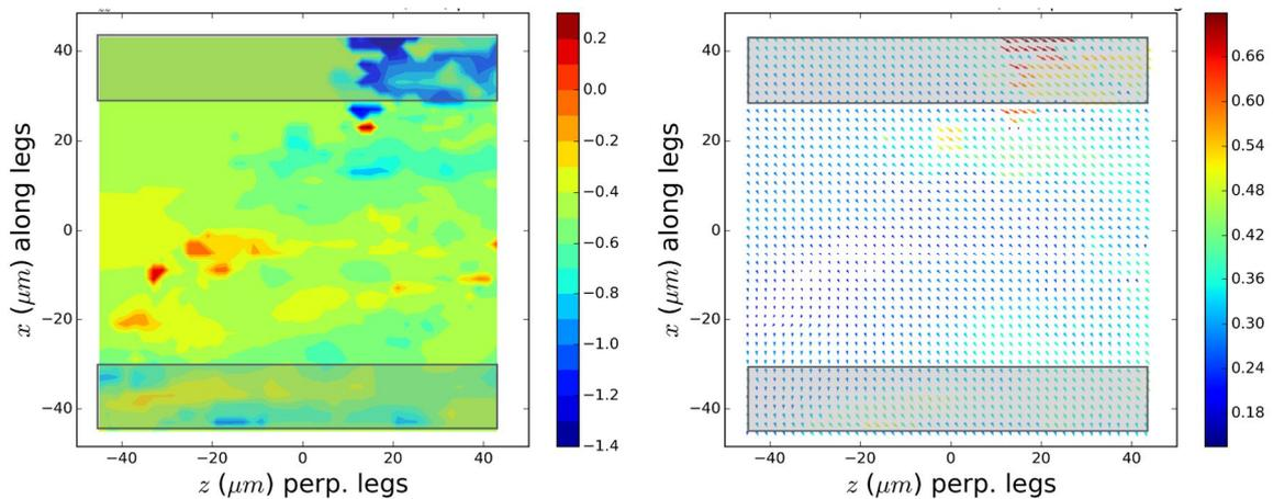
Figure 4: real space distribution of out-of-plane strain (left) and tilt (right) obtained from the reciprocal space maps. Shaded areas show regions where the GaAs membrane sits on top of the piezo legs (part of the bonding area). For this analysis the main maximum in the maps was evaluated and strain is calculated relative to the nominal GaAs peak position.
