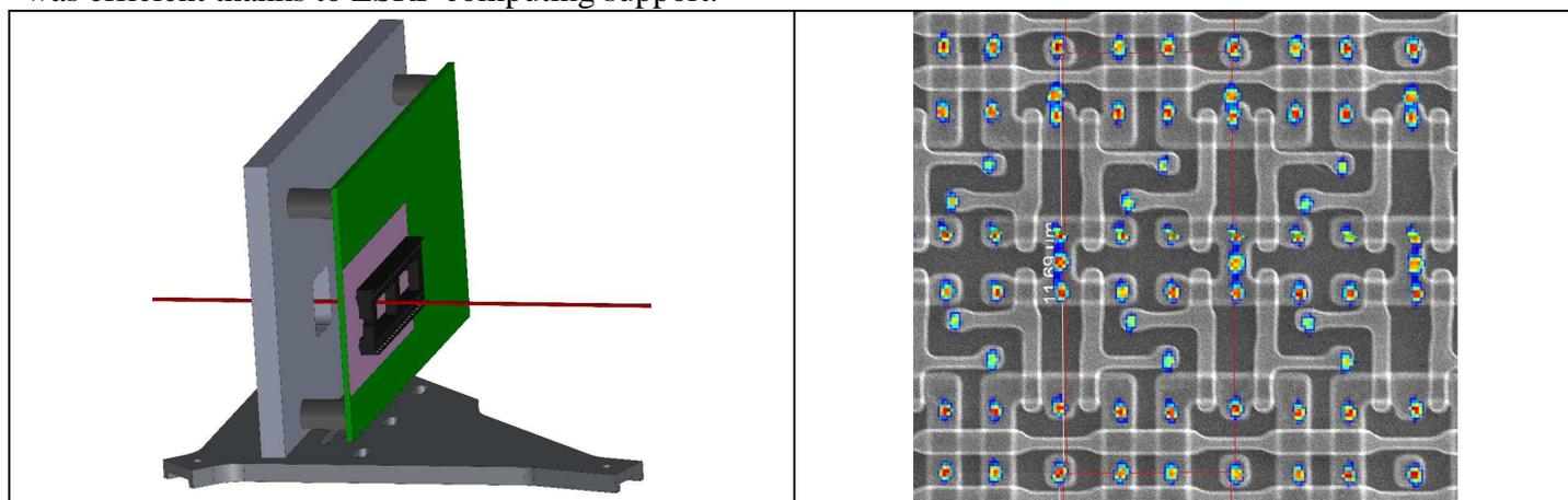
Figure 1 : Geometrical arrangement of the setup (left). Fluorescence map superimposed to the visible light microscope available at the beamline (right) for localization a MEB view of an etched device, showing vias and MOS transistors of RAM cells.
