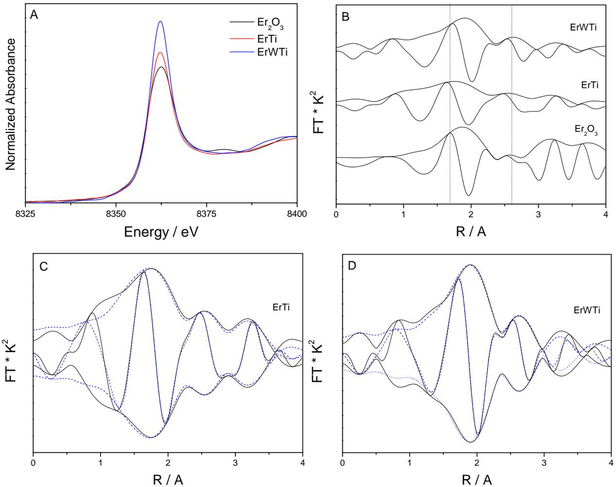
Fig.2. XAS Er  $L_{3}$ -edge results for the  $\text{Er}_2\text{O}_3$  reference and Er-containing single and codoped samples; a) XANES spectra; b) Fourier Transform module and imaginary part of the EXAFS spectra; c and d) Fourier Transform module and imaginary part of the EXAFS signal (full lines) and modelling results (dashed lines).
