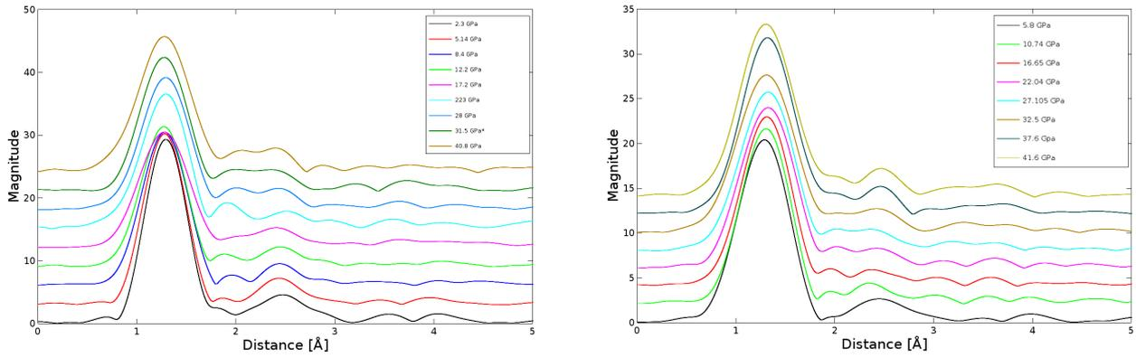
Figure 1: Fourier transform of EXAFS measured at the Ge K-edge at pressures indicated. (left) Ab-Glass; (right) Ab-Di Glass.
