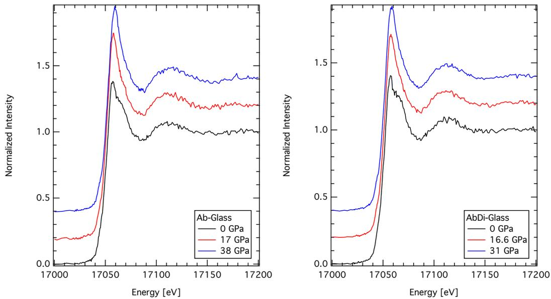
Figure 3: XANES spectra measured at the Y K-edge at the pressures indicated. (left) Ab-Glass; (right) Ab-Di Glass.
