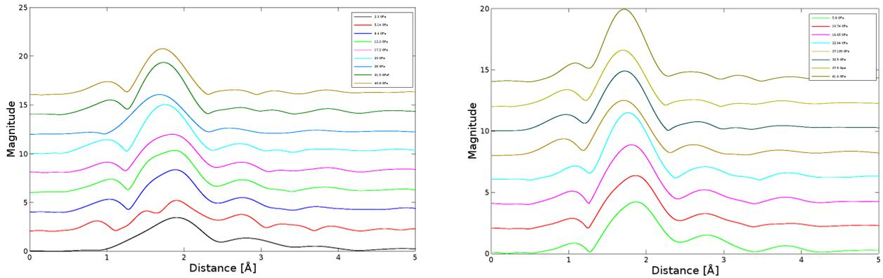
Figure 2: Fourier transform of EXAFS measured at the Sr K-edge at pressures indicated. (left) Ab-Glass; (right) Ab-Di Glass.
