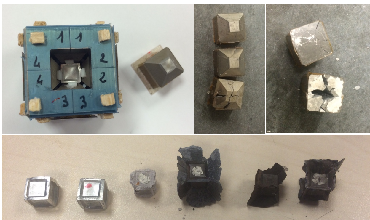
Figure 1: (a) photograph of anvil guide as recovered from test experiment, with deformed Al cube inside. (b) 3 broken secondary anvils, demonstrating the failures emanating from the centre of the deformation truncation. (c) 2 broken anvils, demonstrating the expanding ring crack at the rear-face of the anvil. (d) The recovered experiments: (from left to right) 2 Al cubes, fired pyrophyllite, boron epoxy with gaskets, boron epoxy with no gaskets, boron epoxy with smaller gaskets.
