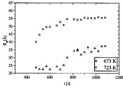
Our aim is to determine activation energy for crystallisation. Today, the interpretation of data is not completely finished. We could show the possibility to observe the phase transition from amorphous to nanocrystalline state in real-time using SAXS.
