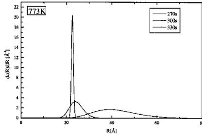
The effect of temperature during crystallisation can be seen in the following figure, where the median of radii is plotted versus time.
