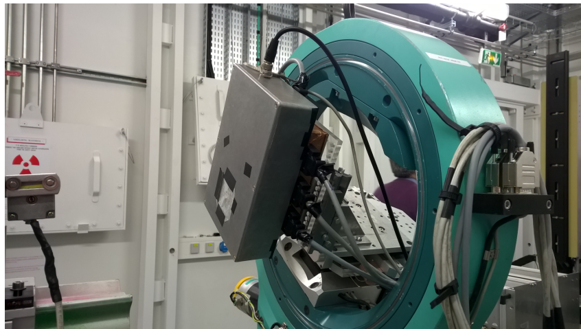
Figure 15 - The detection system mounted on the rotational stage on the XYZ micrometric positioning stages.
