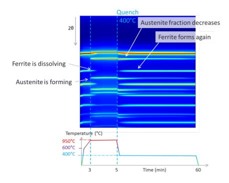
The above graph shows qualitatively the evolution of phase transformations during the different steps of the final annealing. During austenitization at 950°C, ferrite quickly dissolves and a fully austenitic structure is obtained. Immediately after quenching (to 400°C in the presented case), ferrite nucleates and quickly grows, while the residual fraction of austenite stabilizes.
