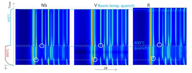
The processes are observed to be similar in the three materials with however some small differences linked to the microalloying content. In order to appreciate better these differences, the diffractograms have been fitted with the Fullprof package to extract variations of phase fractions and lattice parameter.
