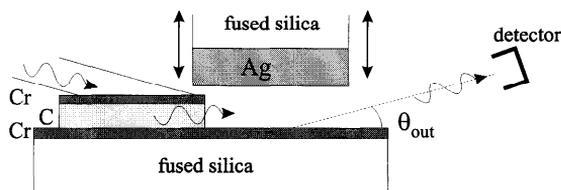
Figure 1b Tunable X-ray waveguide in tandem with a resonant beam coupler (not to scale).
