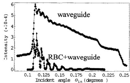
Figure 3 Transmission of RBC and waveguide in tandem compared to transmission of waveguide. Upper curve is shifted 0.1 degree to the right for clarity.
