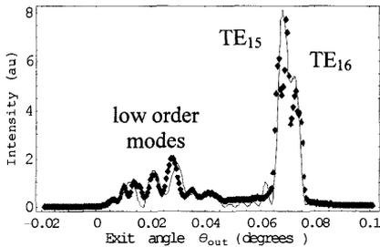
Figure 2 Example Fraunhofer diffraction pattern measured at exit of the waveguide
