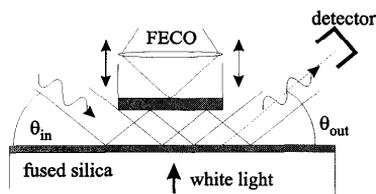
Figure 1a X-ray waveguide with tunable air gap (not to scale).
