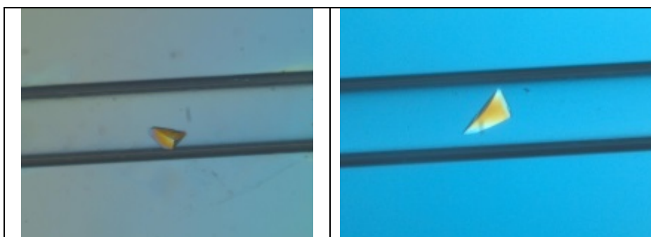
Figure 1. Crystals of McpN-LBD obtained in capillaries of 0.2 mm inner diameter using the capillary counterdiffusion technique.
