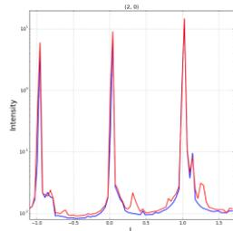
Fig. 2: 1T-TaS<sub>2</sub> (2,0) CTR before (blue) and after (red) 5 min of Cu deposition.
