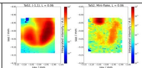
Fig. 4: Real-space map of the integrated intensity for the 1T-TaS<sub>2</sub> (-1,1,0) peak oriented at 0° (left) and 0.1° (right) with respect to the most dominant domain orientation. The two peaks have a different spatial dependence.
