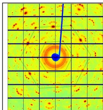
Fig. 1: TSD from 1T-TaS<sub>2</sub> in air, with satellite peaks from CDWs.
