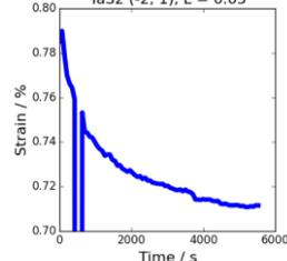
Fig. 3: In-plane tensile strain of the 1T-TaS<sub>2</sub> (-2,1,0) bulk peak during repeated Cu deposition.
