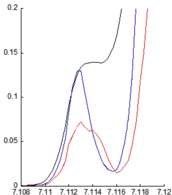
*Figure 1. Comparison of pre-edge region of HERFD-XANES Fe K-edge spectra of four different samples: Fe(II) oxide (black curve), Fe(II) siloxide dimer (blue), Fe(II) grafted on the surface of partially dehydroxylated silica.*
