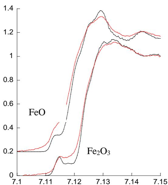
*Figure 2. Comparison of HERFD-XANES Fe K-edge spectra of two standard samples, demonstrating the ability of the method to resolve weak structure. Red spectra belong to the total fluorescent yield (TFY), while black spectra belong to the HERFD data.*
