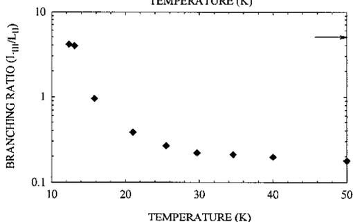
Figure 2: The temperature dependence of the ratio of the  $L_3$  edge integrated intensity to the  $L_2$  edge integrated intensity. The arrow indicates the ratio for  $DyFe_2$  as determined by dichroism measurements [2].
