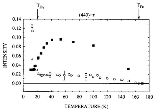
Figure 1: The temperature dependence of the energy integrated intensity of the  $(440)+q$  satellite as measured at the  $L_2$  (8.581keV, open points) and  $L_3$  (7.789keV, closed points) resonant edges of Dysprosium
