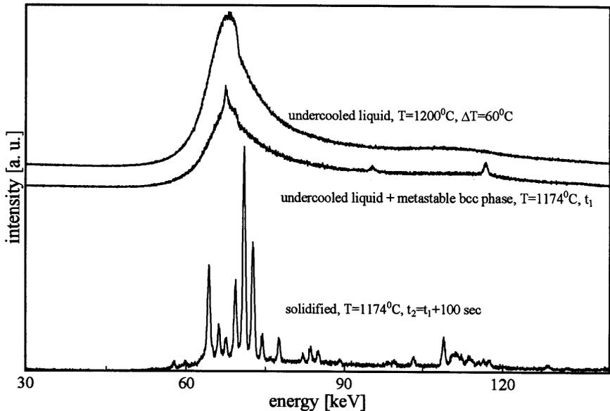
Fig. 1 EDXD spectra of a levitated Ni42V58 sample, measured at different times upon undercooling
