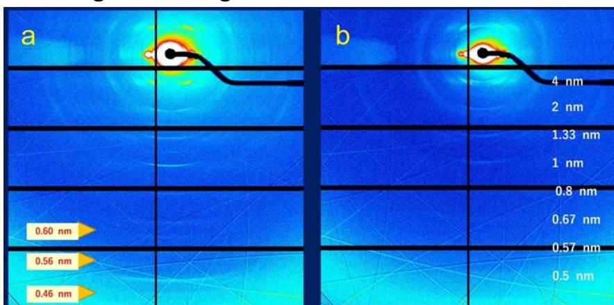
Fig. 1 An example of X-ray fiber diffraction by a WAXS setup. **a** and **b**, diffraction from microtubules without and with paclitaxel, respectively. Numbers on the right side indicate the layer line signals due to approximately 4-nm axial repeat of tubulin within microtubules. Sharp arc lines in the WAXS range are Kossel-Kikuchi lines from the window materials (CDV) we used.
