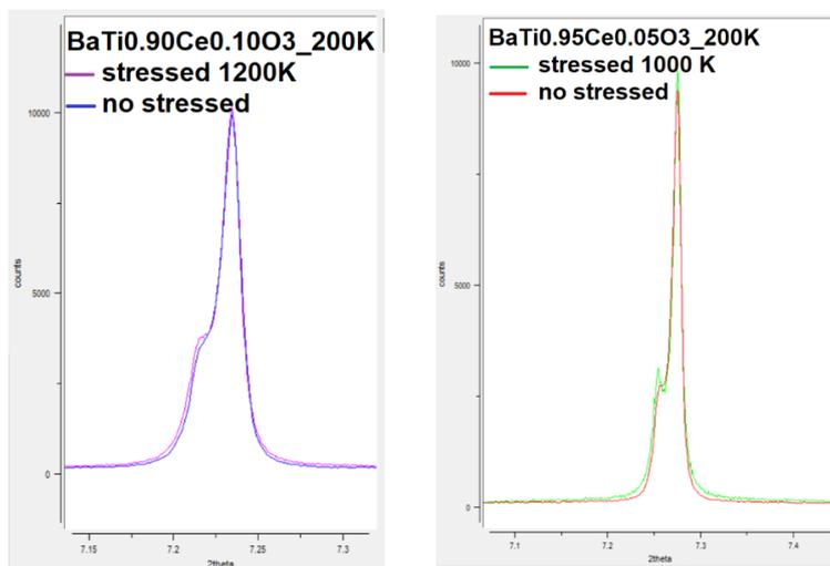
Figure 4. Left panel. Comparison of peak (111) at 200 K for the stressed and no stressed BaTi<sub>0.90</sub>Ce<sub>0.10</sub>O<sub>3</sub>. Peak broadening appears the same for both samples. Data are re-scaled to obtain a fair comparison.
