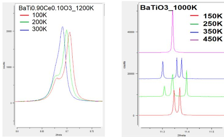
Figure 1. Left panel. Comparison of peak (111) at 100, 200 and 300 K for the BaTi<sub>0.90</sub>Ce<sub>0.10</sub>O<sub>3</sub>. The split clearly visible at 100 and 200 K proves the stability of the rhombohedral phase as well as the shoulder at 300K.
