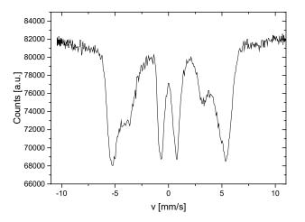
Figure 1 SMS spectrum collected for MgO/Fe/Cr under bias voltage of 10mV.
