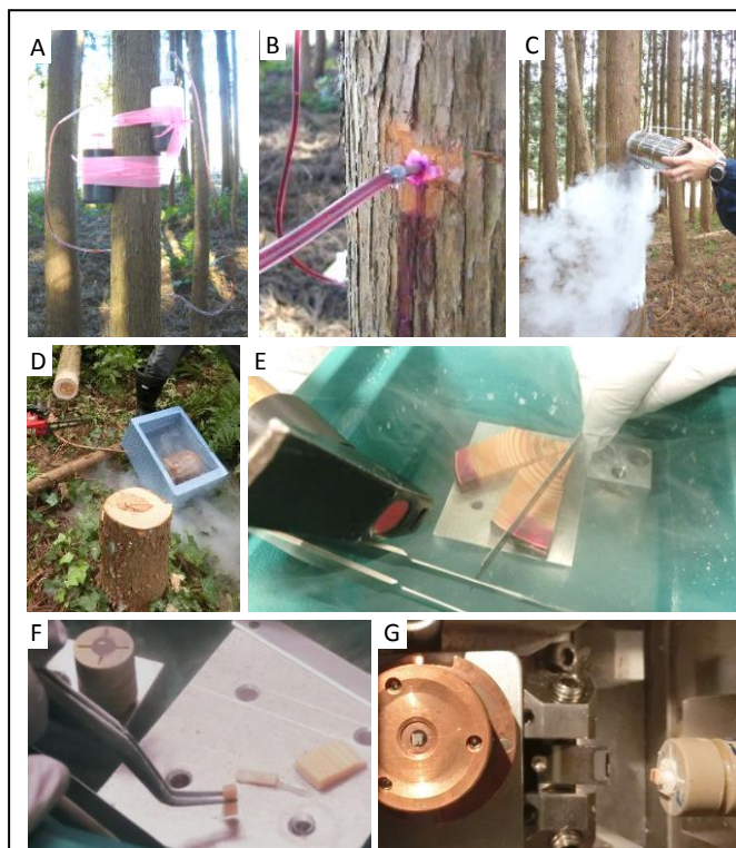
Fig. 1. Schematic drawing of sample preparation. The cesium chloride solution was injected into the trunk of a standing Japanese cedar tree using a stainless tube (A, B). After the injection, the trunk part was freeze-fixed with liquid nitrogen (C), and then the tree was felled (D). A part of the trunk was cut into small pieces (E, F) and subjected to cryomicrotome to prepare thin sections (G). Samples were under frozen state during the entire procedure from the cutting of the standing tree to the end of the analysis.
