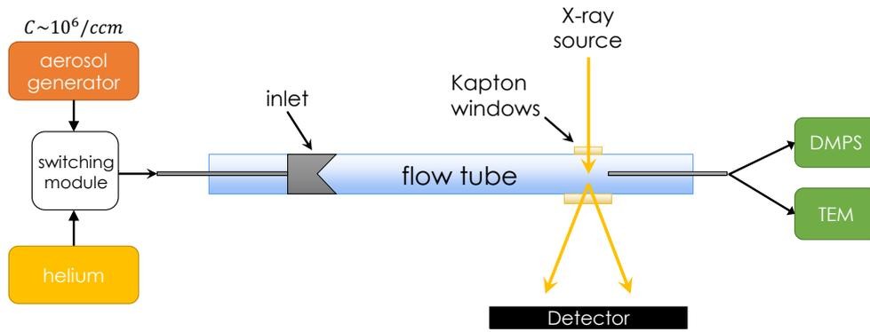
Figure 1: SAXS setup used at the ID-02 beamline for measuring airborne nanoparticles with ultra-low volume fraction.
