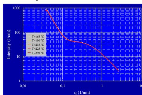
Fig. 2. SAXS patterns recorded *in situ* as a function of the temperature for a pure silica xerogel.
