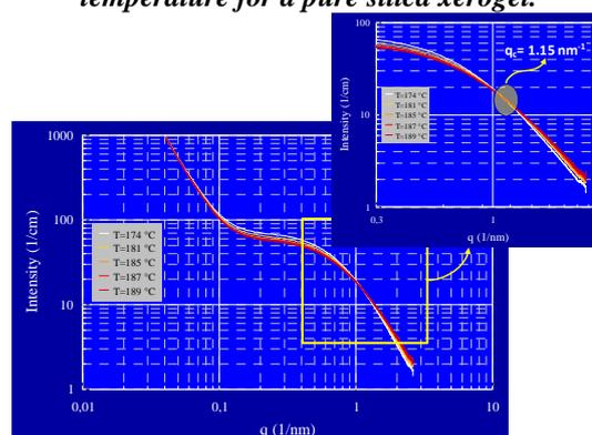
Fig. 3. SAXS pattern recorded *in situ* as a function of the temperature for a xerogel containing 10 at% of tin.
