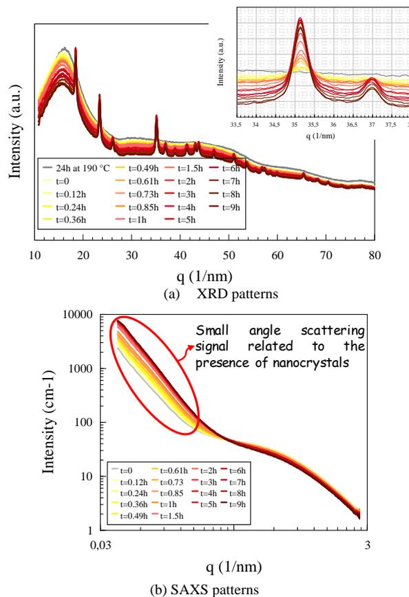
**Fig. 4. Microstructural evolution during isothermal treatment at 350 °C of a xerogel containing 10 at% of tin and previously heat-treated at 190 °C during 24 hours.**
