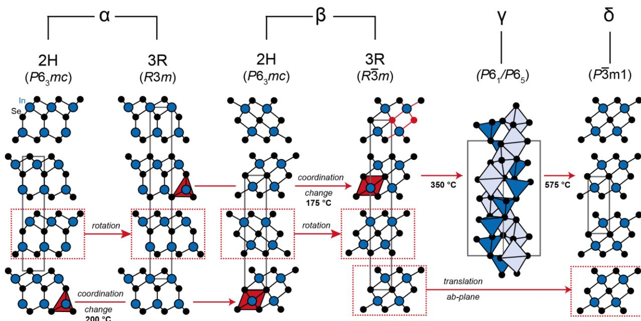
**Figure 1:** Projection of the refined crystal structures of the different  $\text{In}_2\text{Se}_3$  polymorphs. Transition temperatures and symmetry operations between selected polymorphs are indicated.
