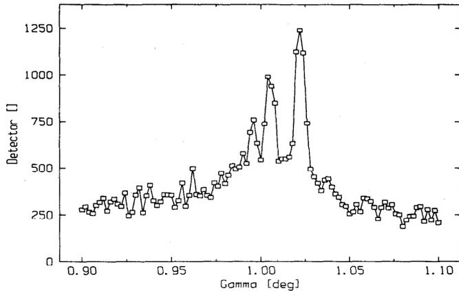
*A detector scan along the gamma (= out-of-plane) direction through a specular reflection of Ge(111). The spikes in the profile resemble a speckle pattern, but no time was available to reproduce these results.*
