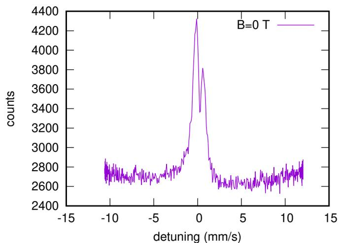
Figure 1: Data set of reflectivity as a function of energy detuning for the cavity structure Pt 3/C 18.5/ $^{57}\text{Fe-SS}$  0.6/ C 22.5/ Pt 15 and incidence angle driving the third cavity mode. Despite zero external magnetic field, the resonance shows a clear electric quadrupole splitting.
