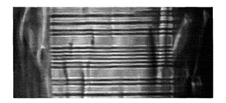
The figure shows a phase-contrast image of LN4 taken at a distance of 12 cm, exposure time 20 s, with the high-resolution CCD camera. The set of strong thick horizontal white lines in the centre of the image correspond to domain walls separated by approximately 2  $\mu$ m as appropriate to a 4  $\mu$ m period array. The images of dislocations, and associated faults in the walls, can clearly be seen crossing the array.
