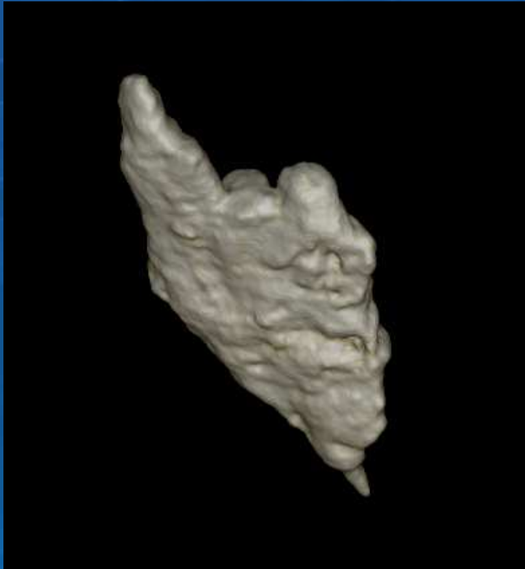
Topotomography of Al grain during recrystallization
