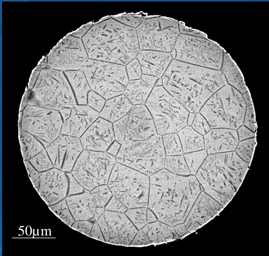
Ti \beta alloy (21s) with \alpha phase precipitates
