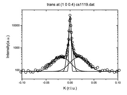
The scan is characterized by a sharp peak and a broad bell shaped foot. The sharp peak is the crystal truncation rod of the Ni substrate whereas the broad peak is the distinct feature of the Cu islands observed even at coverages as low as 0.05 ML.
