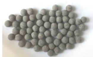
Figure 2. a) Commercial catalyst of \text{Pt}/\text{Al}_2\text{O}_3 provided by Hydrogenious. b) Model catalyst of Pt supported on single crystal \text{Al}_2\text{O}_3 .
