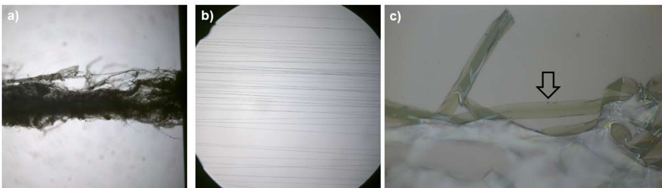
Figure 1 a) Raw Loxosceles web silk stretched on Si 3 N 4 membrane. b) Loxosceles ribbon obtained forced silking of spider, wound several times around metal O-ring. c) Area of Si 3 N 4 membrane with deposited Loxosceles ribbons. The arrow indicates a flat ribbon of about 8 \mu m diameter and 50 nm thickness.
