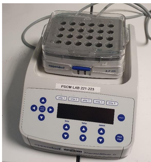
Figure 2. Temperature controlled shaker that was used for samples with slow degradation kinetics. pH in the eppendorf tubes was regularly measured and adjusted, if needed. Samples could be taken out for SAXS measurements and then put back into the tubes.
