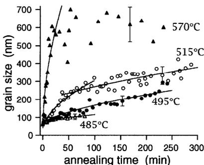
FIG. 1: Grain growth in nanocrystalline Fe measured by diffractometry. Solid lines are fits of a parabolic growth law ( $n = 2$ ).
