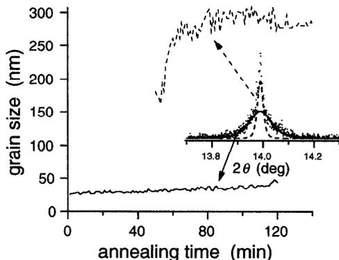
FIG. 2: Grain sizes in nanocrystalline Pd annealed at 355°C. Inset shows (111) peak along with narrow and broad component fitting functions.
