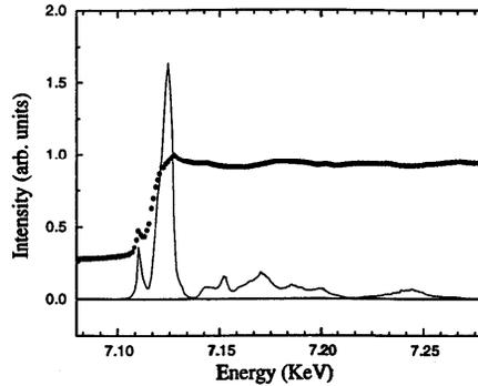
**Figure 1.** Energy dependence of the intensity of  $(002)_c$  reflection near the iron K-absorption edge at  $T=20$  K. Closed circles represent the measured fluorescence.
