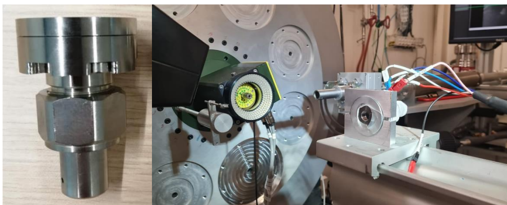
Figure 1 – Optical cell used for the operando XRD experiment (left) and experimental configuration at the beamline (right).
