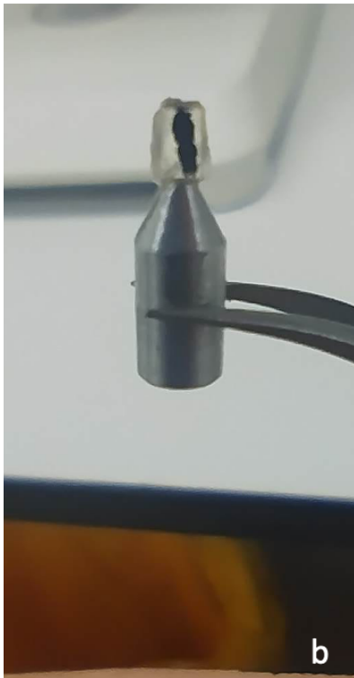
Figure 1. Sample selection and setup. a) MicroCT of the selected specimen. b) Re-embedding and mounting of the selected specimen on the beamline-compatible aluminium stub. c) resin was further trimmed, and stub placed in the beamline holder; d) sample entering the beamline chamber.
