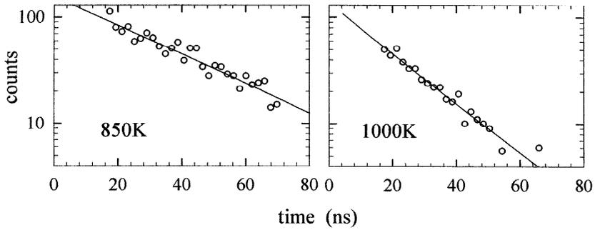
Fig. 1. Decay of SR intensity scattered from the crystal plane  $(220)$   $\text{Fe}_3\text{Si}$  at 850K and 1000K.
