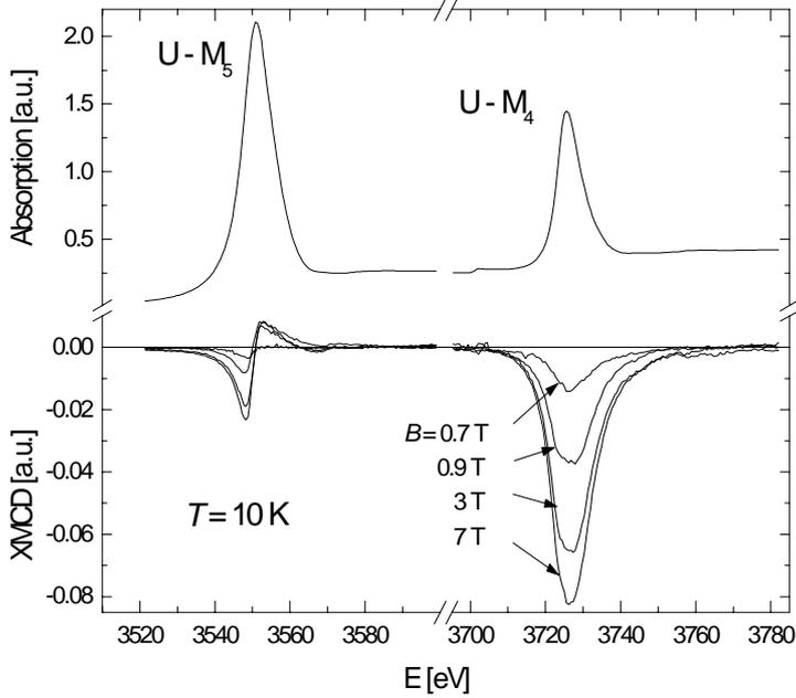
Fig. 1. Uranium  $M_{4,5}$  absorption and XMCD spectra of UCoAl single crystal measured along the  $c$ -axis at different fields.
