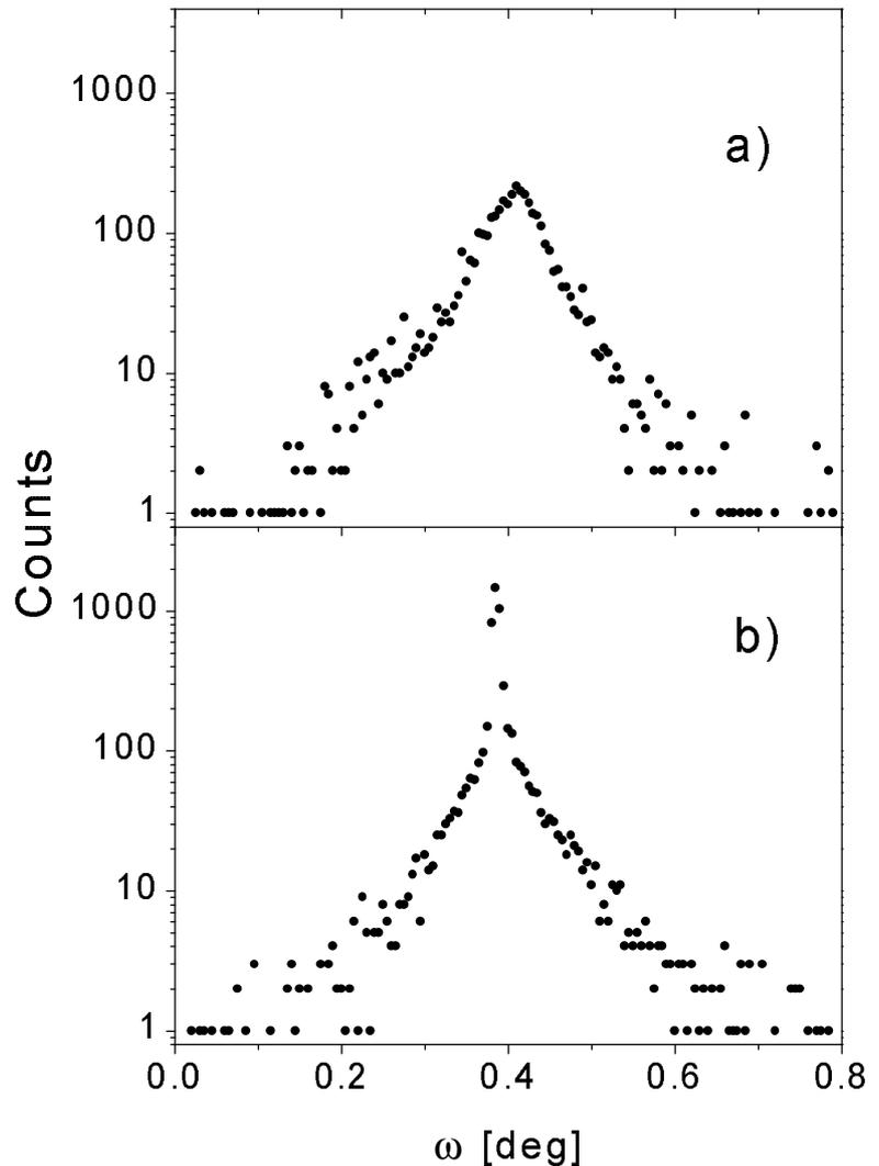
Fig. 1. Off-specular SMR scans at the AF reflection of a MgO(001)/[ $^{57}\text{Fe}(25\text{\AA})/\text{Cr}(14\text{\AA})$ ] $_{20}$  ML: a) small-domain state, b) large-domain state.
