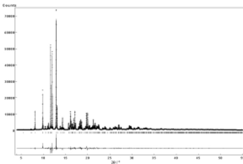
Fig. 1. (on the left) The temperature evolution of the diffraction pattern of HFC-134a shows the solid-solid phase transition at about 112 K on cooling.
