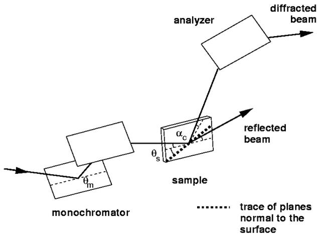
Fig. 1. Sketch of the optical geometry used at the ID01 beamline for surface diffraction.
