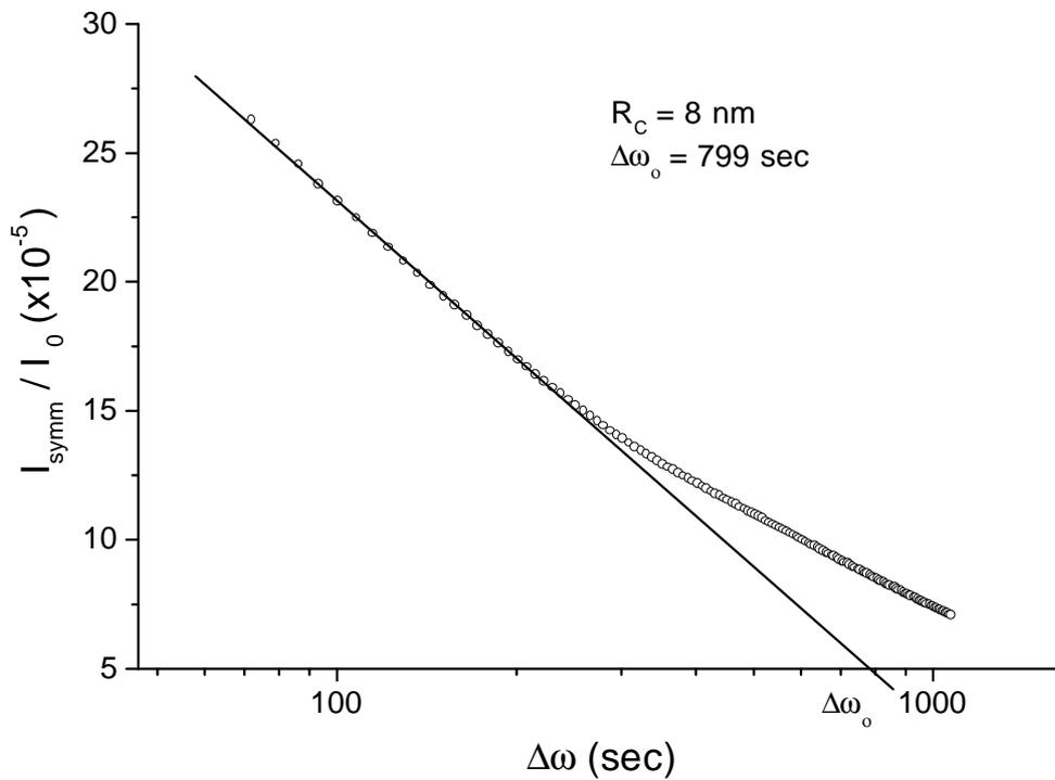
Fig. 3. Symmetric part of DXS vs sample rotation angle. From the intercept of the straight line on the angular axis, the cluster radius is obtained.
