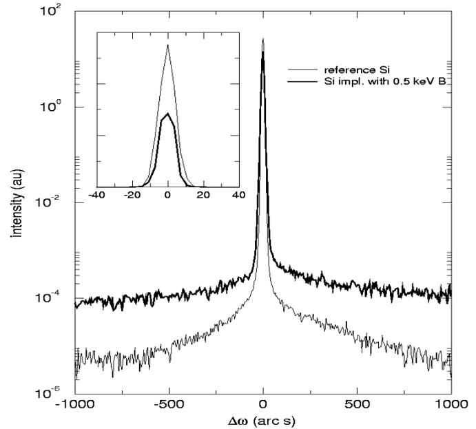
Fig. 2. Intensity profiles obtained from  $\{220\}$  planes normal to the surface of a 0.5 keV B implanted Si (thick line). The profile of an unimplanted reference Si is also reported.
