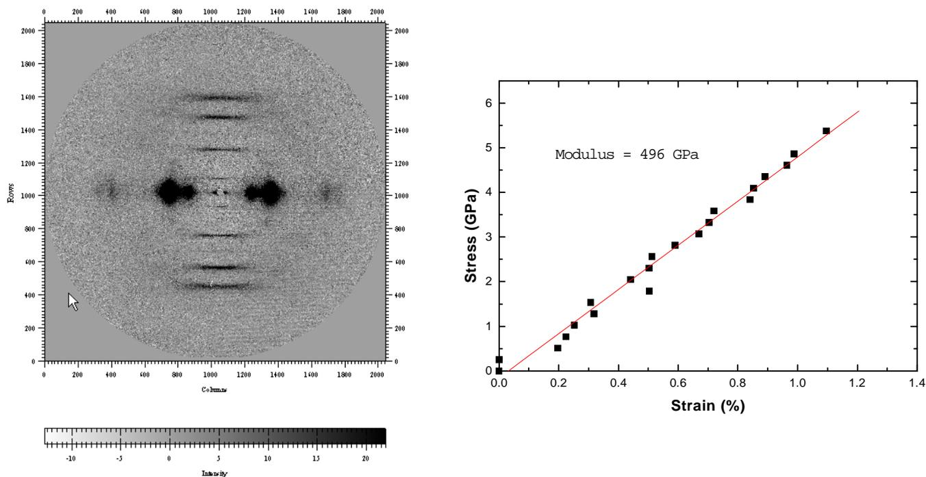
*Figures 1 & 2: Diffraction pattern of PBO, and the calculated crystal modulus*
