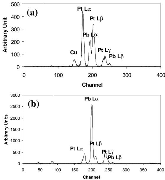
**Fig. 2:** Fluorescence spectrum for 200 nm PZT film on Pt. (a) using the initial setup in the cryostat; (b) the final measurements in grazing angle. The Pt L peak intensity is reduced and the intensity of the Pb L peak is enhanced.
