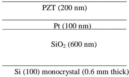
**Fig. 1:** Schematic cross section of the samples.
