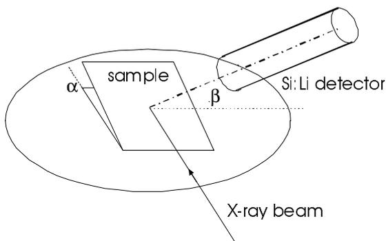
**Fig.3:** Schematic setup of the fluorescence measurement in grazing angle incidence.
