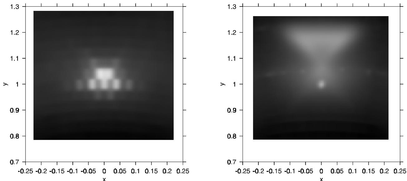
Fig.3 Mapping around (0 1 0.12) of clean Au(111) (a) and of 6ML Fe/Au(111) (b)
