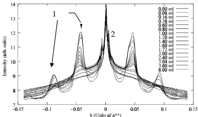
Fig.2 High resolution angular scan through the reconstruction peaks in the vicinity of the (0 1 0.12) truncation rod
