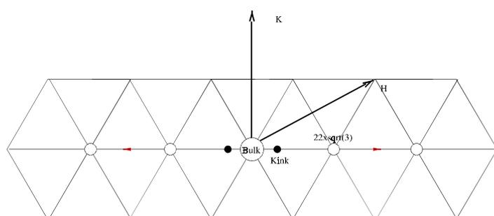
Fig.1 Reciprocal space of the Au(111) reconstructed surface. Large open circles: bulk in-plane periodicity. Small open circles:  $22\times\sqrt{3}$  reconstruction. Small solid circles: herringbone reconstruction.
