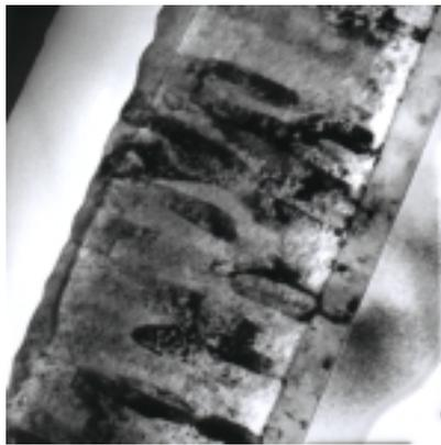
Fig. 1: FeCo single layer with Ti bond coat on the Si-substrate the columnar grains grew through the whole layer [N. Wanderka, M. Macht HMI Berlin]
