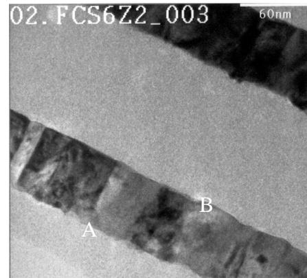
Fig. 2: Columnar layer growth of FeCo-/SiO<sub>2</sub> multilayer FCS6Z2 (A = FeCo-SiO<sub>2</sub> interface, B = SiO<sub>2</sub>-FeCo interface) [N. Wanderka, M. Macht HMI Berlin]
