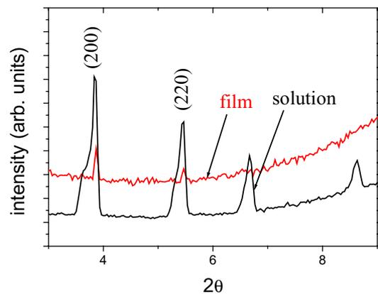
**Fig. 2** Radial ( $2\theta$ )-scans of LTA zeolite in solution (black) and on glass plate (red) in the  $2\theta$  range  $3-10^\circ$ .
