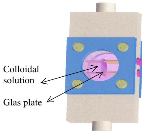
**Fig. 1.** Container for in-situ X-ray measurements of zeolite crystal growth.
